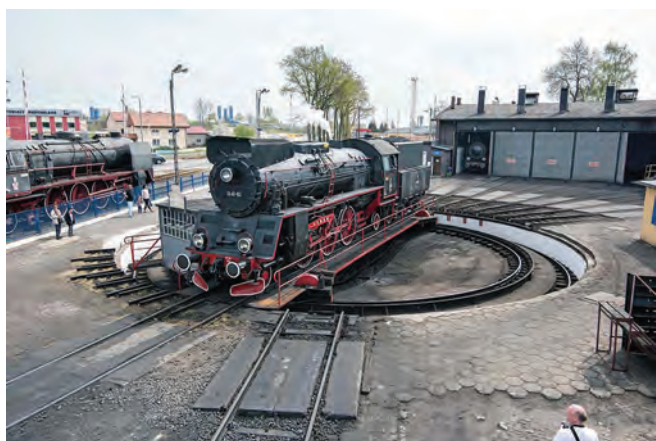
Loco 0149-69 being turned prior to being refuelled with coal and water. Made at the Fablok - Chrzanów workshops in 1949
